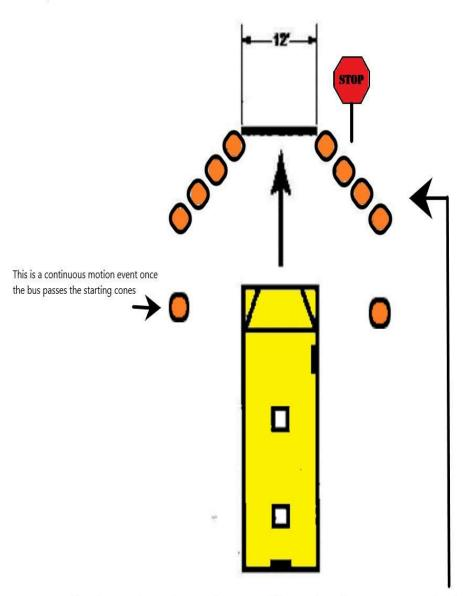
There is no set distance between the cones and the stop line. All measurments are taken from the bumper to the front edge of the stop line. Student crossing arms are not part of the measurment.
