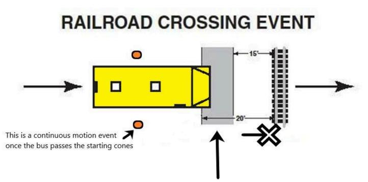
Gray highlighted area indicates the 5' measuring zone Distance marks are **NOT** marked on the course prior to event starting
